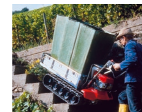
The HP 500 power carrier has traction, even on a slope
